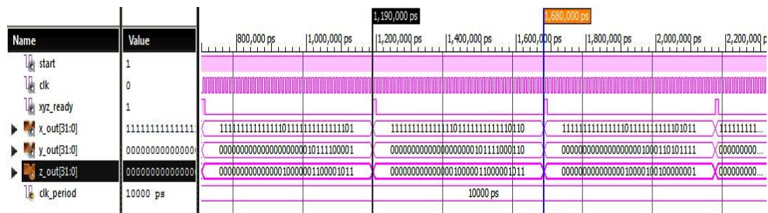
Fig. 5 Xilinx ISE simulator results of the Heun-based PC chaotic oscillator unit.
