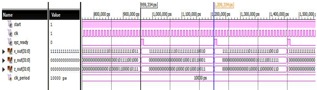
Fig. 4. Xilinx ISE simulator results of the Euler-based PC chaotic oscillator unit.
