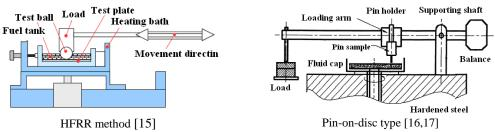
Fig. 1. Schematic diagram of wear testing rigs.
