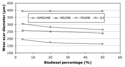
Fig. 2. Effect of biodiesel percentage on lubricity.
