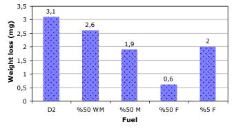
Fig. 4. The weight loss of the samples worn in the pin-on-disc type abrasion machine.
