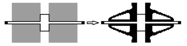
**Figure 4.** A frequency gap maximization topology optimization problem [11] of a compliant inertial amplification mechanism [12].
