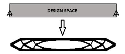
Figure 3. A fundamental frequency maximization topology optimization problem [10].
