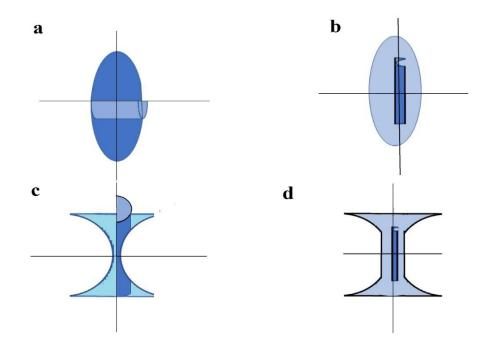
**Figure 4.** Illustration of spherocylindrical lenses used in the correction of complex refractive errors; lens in a is (+,+), lens in b is (+,-), lens in a is (-,+), lens in a is (-,-).
