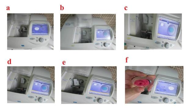
**Figure 11.** Figure illustrates lens placement (a), grinding (b), smoothing (c), polishing (d), edge cleaning (e) processes and the final product (f).
