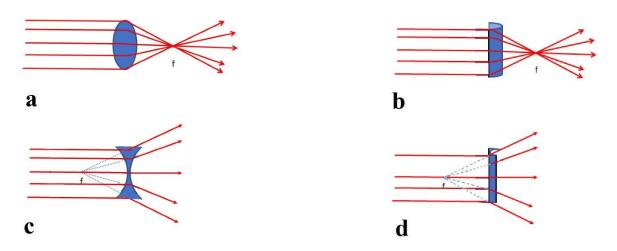
**Figure 3.** Illustration of spherical convex with (+) dioptre (a), cylindrical convex with (+) dioptre (b), spherical concave with (-) dioptre(c), cylindrical convex with (-) dioptre.
