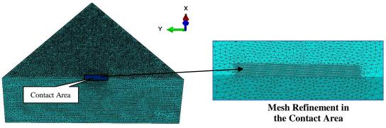
Figure 4: Created FE model and mesh refinement
