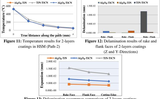
Figure 13: Delamination occurrence comparison of 2-layers coatings
