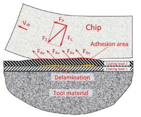
Figure 3: Delamination formation between multi-layer coating layers [28]
