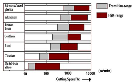
Figure 1: High-speed cutting scales based on workpiece materials being machined [8]
