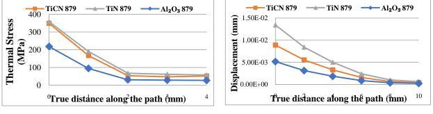
**Figure 8:** Thermal stress results for each coating material in HSM operation (Path-3)
