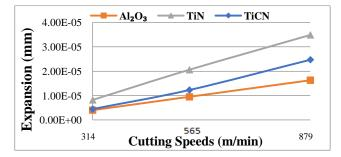
Figure 10: Maximum thickness expansion (in Z-Direction on the rake faces)
