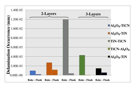
Figure 17: Delamination comparison in multi-layer coatings on the rake and flank faces (Z and X-Directions)
