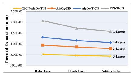
Figure 16: Dimensional thermal expansion comparison of multi-layer coatings
