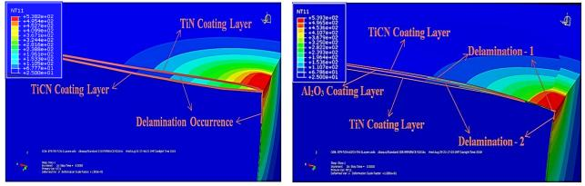
**Figure 14:** Cross-sectional view cut along the rake face of TiN-TiCN 2-layers coating to illustrate delamination existence in HSM
