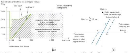
Figure 10 LVRT requirement for (a)the offshore grid connection (b) for the offshore grid connection at the converter level by TenneT [8]
