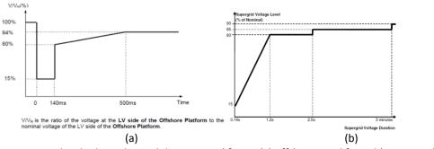
Figure 9. Fault ride through capability required for an (a) offshore wind farm, b) OFTO in the UK [9]
