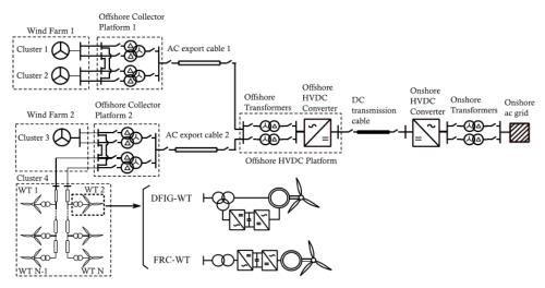
Figure.1.General configuration of an OWPP with two wind farms connected through an HVDC point-to-point link [4]
