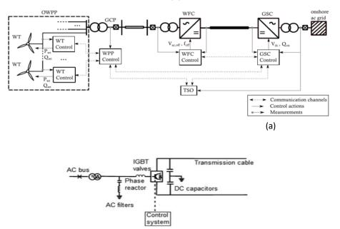
(b) Figure.2. (a) General control scheme of a HVDC-connected OWPP [5] (b) VSC HVDC transmission system [2]
