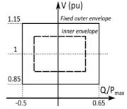
Figure 3 : ENTSOE requirements for voltage at the grid connection point of a dc-connected system [7]
