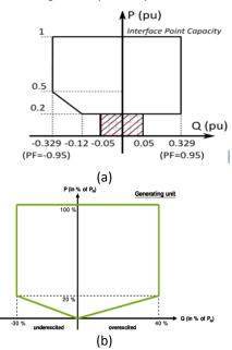
Figure 4 (a) National Grid (Great Britain) requirements for reactive power capacity at the interface connection point of a WPP or a DC-connected system [11], (b) "Offshore": Minimum requirements for the P/Q-operation range of a generation unit within the voltage range of +/- 5 % UN (at the generation unit) by TenneT[8,9]
