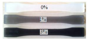
Figure 2. With and without ash added plastic material samples
