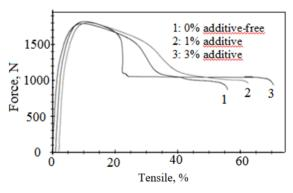
Figure 6. Tensile-Force Diagram applied on three different sample
