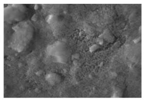
Figure 4. SEM images of the plastic material produced by adding 1% ash, 100000x
