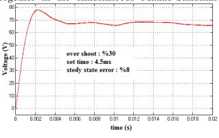
Figure 4. For %60 duty input voltages, T(s) and power system outputs
