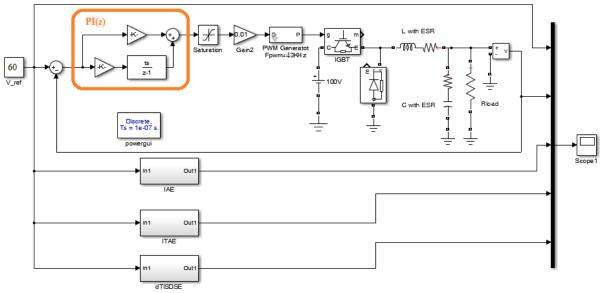
Figure 12. 4 control systems with 4 different controller's parameters
