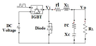
Figure 2. Buck converter topology
