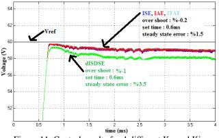
Figure 11. Control results for 4 different Kp and Ki parameters
